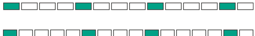
Equidistant (bottom) generates exactly uniform cell spacings, while with CBR (very bottom), the average spacing is the same.
